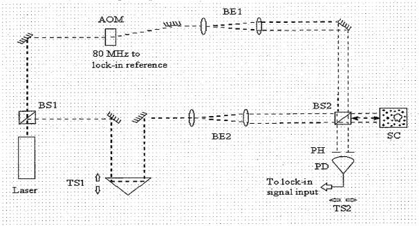
Thus, by changing the length of the delay arm of the interferometer (see the figure above), images may be formed for different depths within the sample. The photons detected would be those that traveled ballistically to the object, reflected back, and traveled ballistically to the detector. Depth resolution will be limited primarily by the coherence length of the laser. And, the
